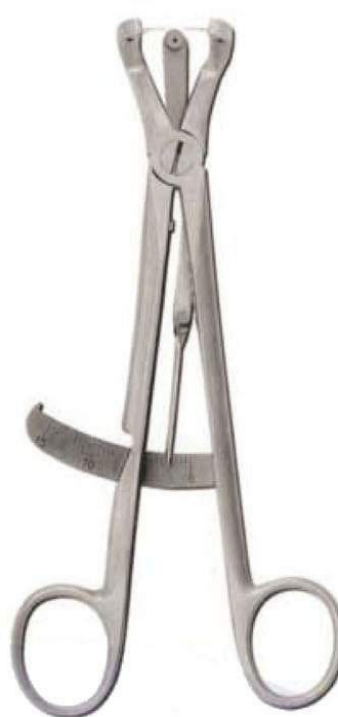
JI-1280 Bone Thickness Gauge 40mm, 180mm
